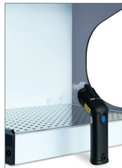
Flow demonstrated with a Dräger Flow Check.
